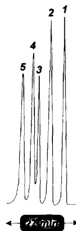
Fig. 3. Chromatogram of a mixture of aromatic hydrocarbons. Packing: as in Fig. 2. Column temperature: 150.2°C; argon carrier gas flow-rate: 20.7 ml/min. Peaks: 1=benzene; 2=toluene; 3= ortho -xylene; 5=ethylbenzene; 6=propylbenzene.
